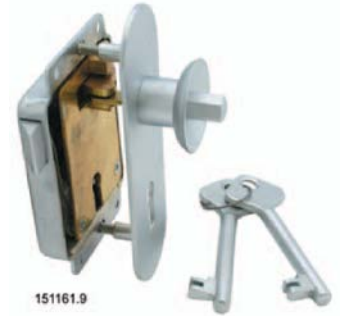
#21.512 Push pin Latch with 30 mm backset with round cylinder key lock Case 55 x 78 mm. For door thickness from 5/8" to 1 3/16"
